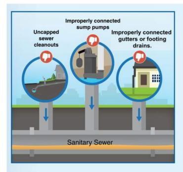
**Inflow** is clear water that quickly enters the wastewater system after rainfall events from sources such as sewer cleanouts, sump pumps, gutters, building foundation drains, and broken maintenance hole covers.
